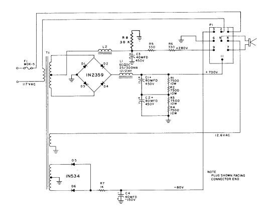
Figure 1. NCX-A Power Supply Schematic
