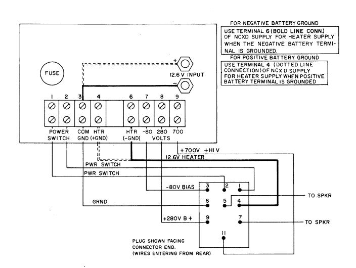
Figure 3. NCX-D Wiring Connections
